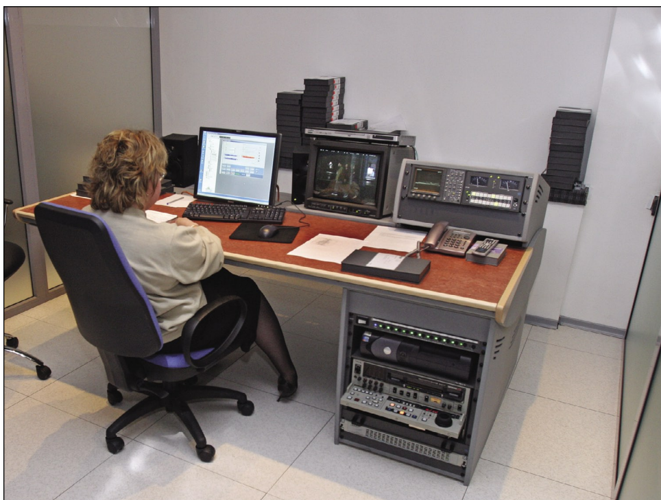
At the ingest position, analog Betacam tapes are encoded and checked for quality.
