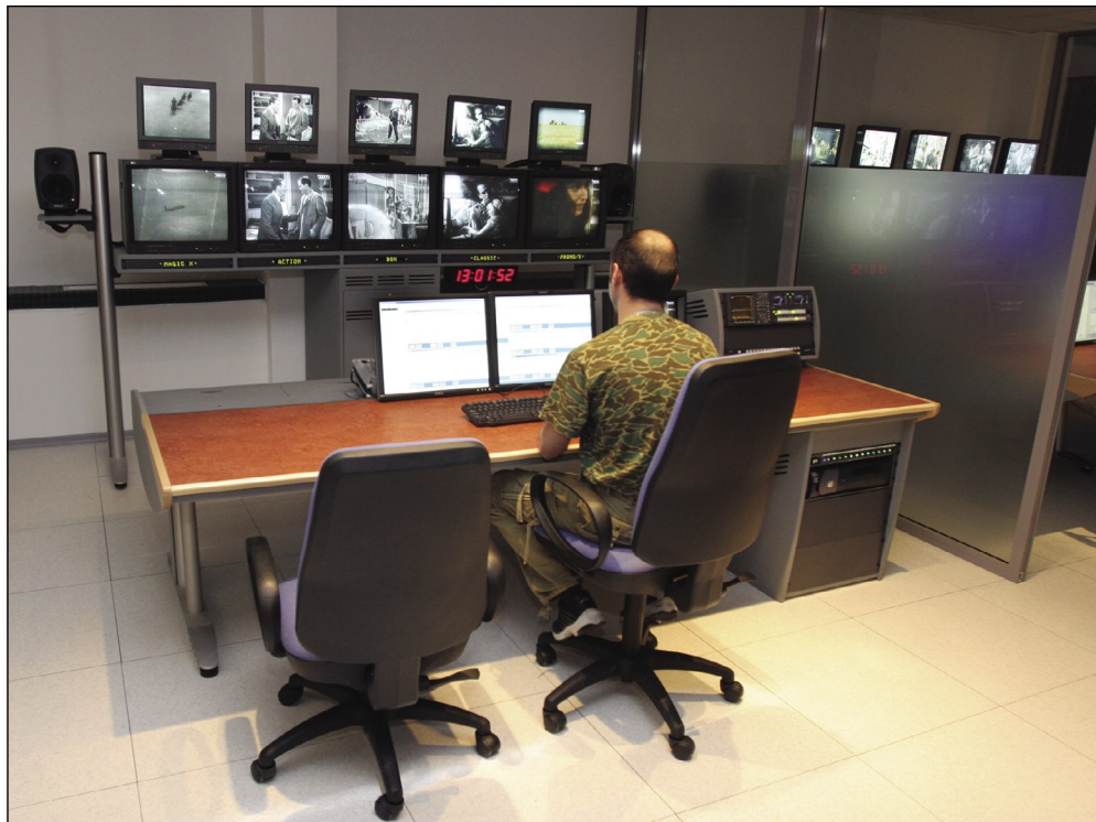
In Playout 2, an operator uses a dual-head playback client for the Pebble Beach Neptune automation system to run five channels.
